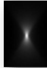
Figure 2. Dose distribution recorded on radiographic plate using CONVERAY technology
